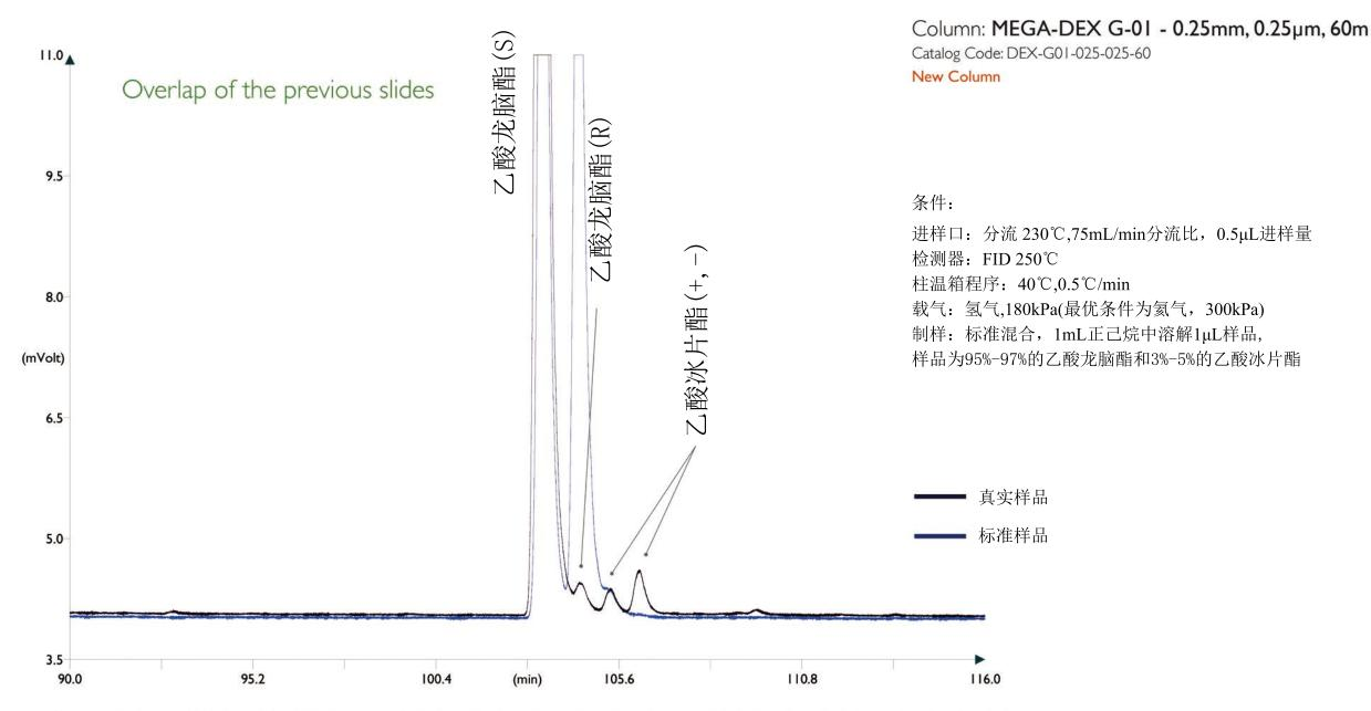
This separation is very difficult to obtain, for this it is recommended to follow the chromatographic conditions here reported, which are the optimized parameters for this analysis.
